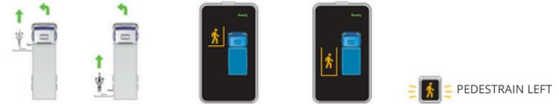
④ When a VRU is detected within 1m vertical distance from the nearside, led display shows a red icon and a pillar led indicator shows a red warning.
