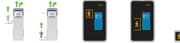
③ When a VRU is detected within 1.1m to 2.2m vertical distance from the nearside, left turn signal is not used. Only use GYRO to detect left turning. No audio alert when VRU is within 1.1m To 2.2m, just yellow icon, the display shows a yellow icon in the corresponding position, and left A-Pillar led indicator gives a yellow flashing.
