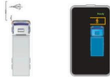
③ Speed at 0 < speed ≤ 5km/h, when VRU are detected in front of the vehicle, the display shows a red icon and gives audio warning.
