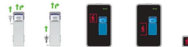
⑤ When a VRU is detected within 1.1m vertical distance from the nearside, left turn signal is not used. Only use GYRO to detect left turning. The led display shows a red icon and audio warning, A pillar LED gives a red flashing warning.
