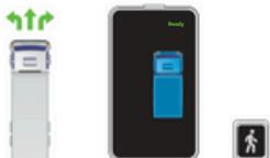
② When a VRU is detected within 1m to 2.2m vertical distance from the nearside, the display shows a yellow icon in the corresponding position, and left A-Pillar led indicator shows a yellow icon warning, and no audio warning.
